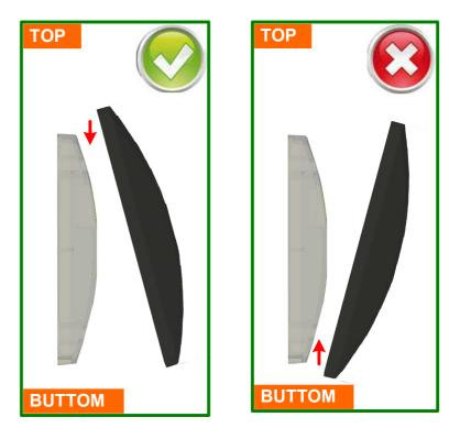
Above picture shows the correct direction (TOP) that outer housing needs to be applied.
