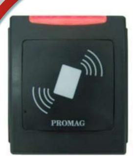
Frequency: 13.56MHz Interface: RS232, Wiegand, ABA TK2 Card Types: ISO 14443A/B ISO 15693 INSIDE PicoTag DC Power: 12V /160mA@12V Temperature Range: *Operating Temp:* -10°c ~ +60°c Humidity: 10%~ 90% relative Dimensions: 105(L) x 105(W) x 20.74(D) mm Weight: 320g
